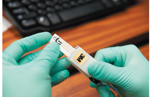
A sensor that can detect toxic chemicals is connected to a cable in the lab. (Peter Morenus/UConn Photo)
